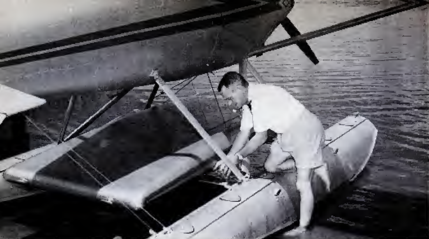
Boat is quickly detached from plane. Shaped like an airplane wing, it provides added lifting force in flight
